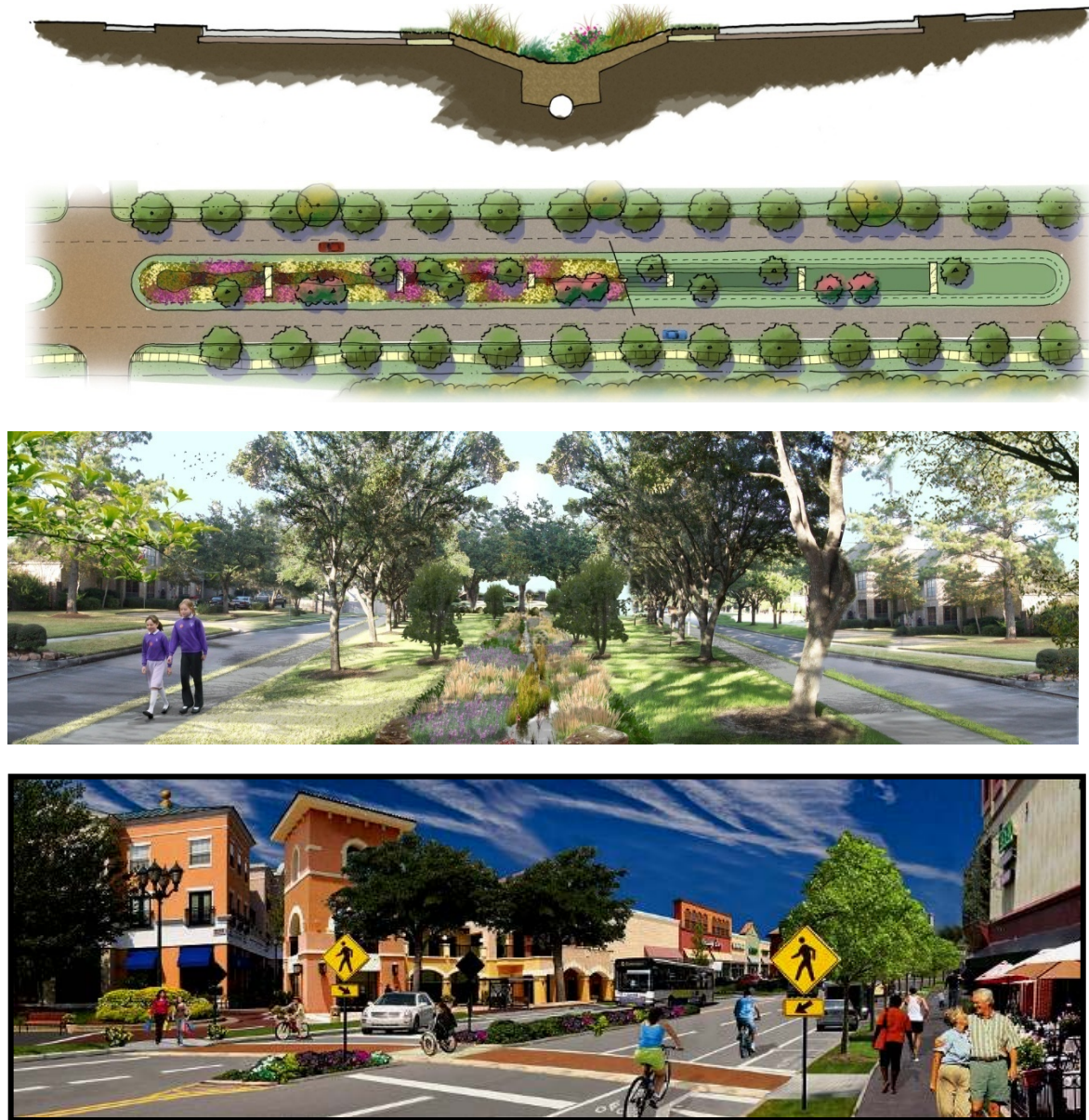
Figure 3.8 – Examples of center median infiltration/filtration systems
